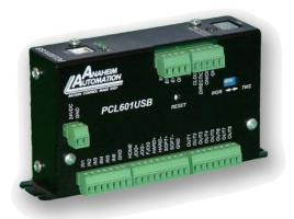
The PCL601USB step motor controller provides independent programming of acceleration/deceleration, base speed (start up speed), max speed (running speed), jog speed, and the number of steps to be taken in both relative and absolute positioning modes. On absolute positioning moves, the PCL601USB automatically determines the proper direction to go and the number of steps to take. The relative positioning will move a number of steps in the direction that the user defines.
